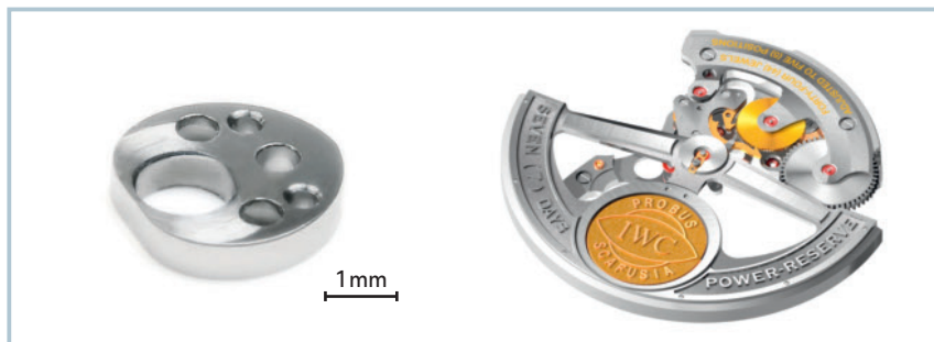
4 A hole is made in the ›hammer‹ (left) to a final diameter of 1.296 mm, accurate to within 2 µm. The hammer forms part of the ›Pellaton‹ watch winding mechanism (right)
