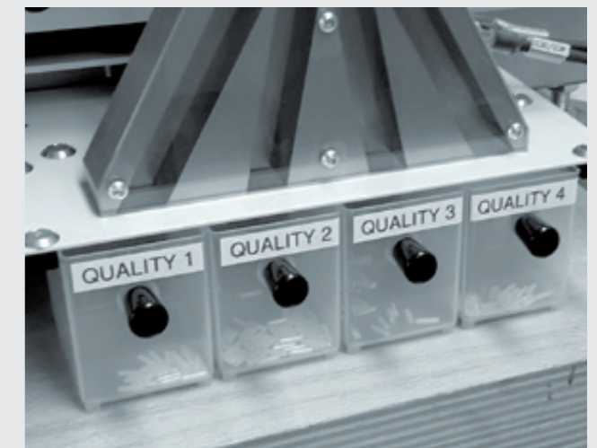
After measuring the work pieces are sorted into 4 quality classes
