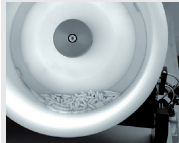
The workpieces are filled into a drum feeder and led to the handling station
