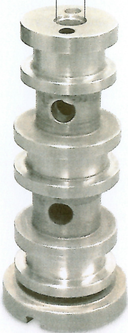
4 The MBS easily provides the high level of accuracy required when processing this sliding sleeve with cross bores for hydraulic applications (Photo: Microcut)
